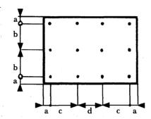
(b) Devices for illuminating a wide plate (520  $\times$  120 mm)
