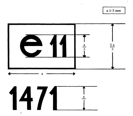
The device bearing the EEC component type-approval mark shown above is a rear registration plate lamp EEC type-approved in the United Kingdom (e 11) under the number 1471.
