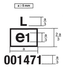
The device bearing the EC component type-approval mark shown above is a rear registration plate lamp, type approved in Germany (e1) pursuant to this Directive (00) under the base approval number 1471.
