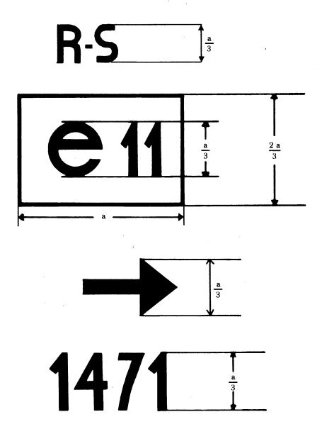
The device bearing the EEC type-approval mark shown above is a device comprising both a rear position (side) lamp and a stop lamp, EEC type-approved in the United Kingdom (e 11) under the number 1471. The arrow means that, on the side to which it points, the photometric specifications are satisfied up to an angle of  $80^{\circ}$  H.
