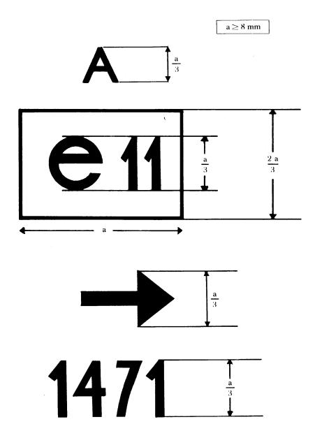
The device bearing the EEC component type-approval mark shown above is a front position (side) lamp, EEC type-approved in the United Kingdom (e 11) under the number 1471. The arrow indicates the side on which the photometric specifications are satisfied up to an angle of  $80^{\circ}$  H.
