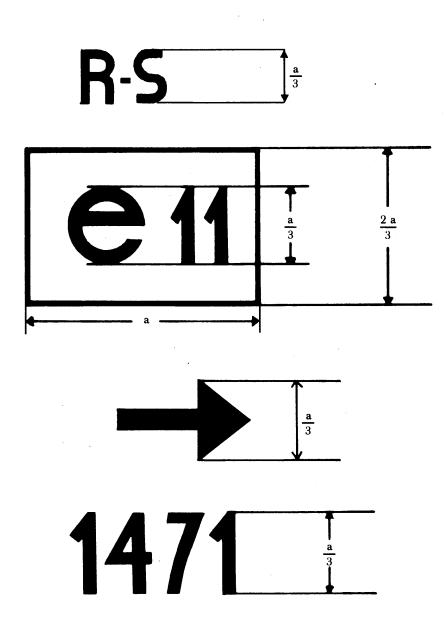
The device bearing the EEC type-approval mark shown above is a device comprising both a rear position (side) lamp and a stop lamp, EEC type-approved in the United Kingdom (e 11) under the number 1471. The arrow means that, on the side to which it points, the photometric specifications are satisfied up to an angle of  $80^{\circ}$  H.
