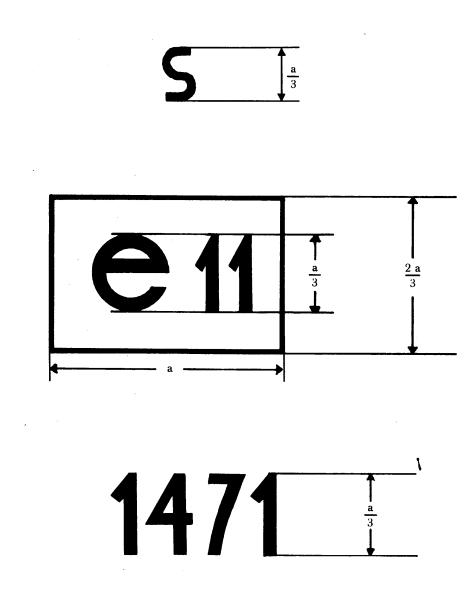
The device bearing the EEC type-approval mark shown above is a stop lamp, EEC type-approved in the United Kingdom (e 11) under the number 1471.
