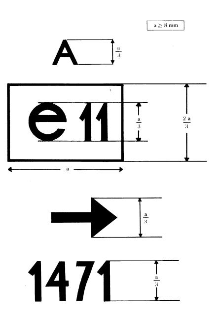
The device bearing the EEC component type-approval mark shown above is a front position (side) lamp, EEC type-approved in the United Kingdom (e 11) under the number 1471. The arrow indicates the side on which the photometric specifications are satisfied up to an angle of  $80^{\circ}$  H.
