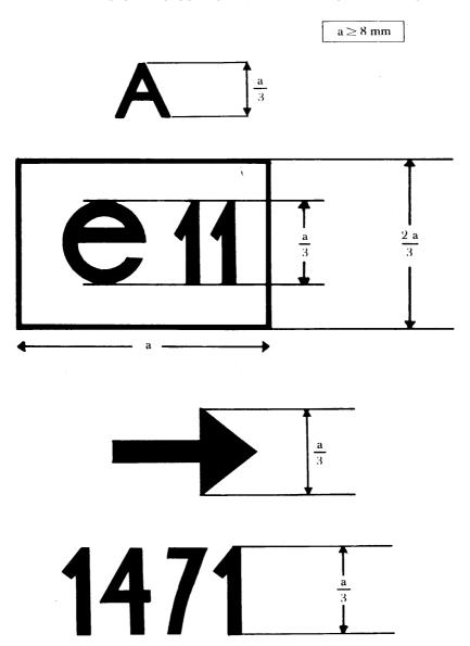
The device bearing the EEC component type-approval mark shown above is a front position (side) lamp, EEC type-approved in the United Kingdom (e 11) under the number 1471. The arrow indicates the side on which the photometric specifications are satisfied up to an angle of  $80^{\circ}$  H.
