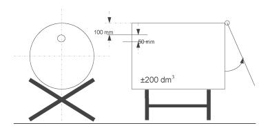
(d) On a 200 × 200 mm metal support place a paraffin wax candle 20 to 40 mm in diameter and 100 mm high. The candle shall be replaced when having a height of less than 80 mm. The candle's flame is protected from the action of the spray by a 150 mm wide, 200 mm high deflector. This includes the plane inclined at 45° produced 150 mm from the base of the deflector (Figure 6.3.2.2.);
