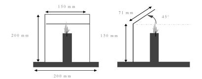
(e) The candle placed on the metal support shall be positioned midway between the two ends of the drum (Figure 6.3.2.3);
