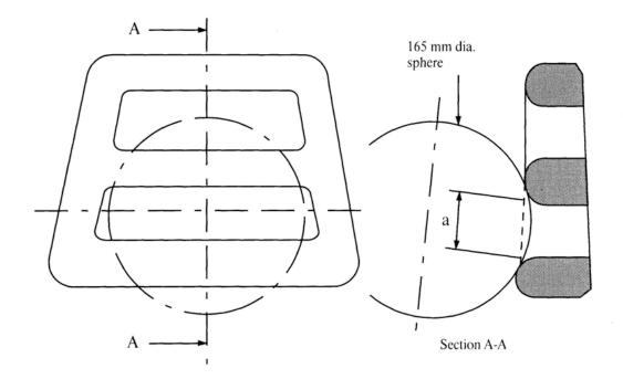
*Note:* Section A-A is to be made in a point of the gap area which allows the maximum sphere intrusion without exerting any load.
