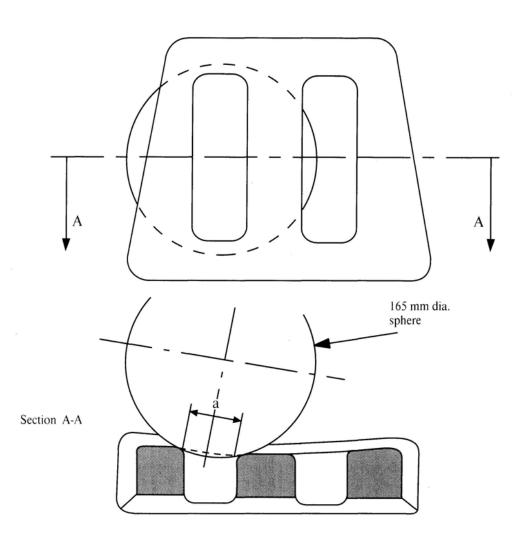
*Note*:Section A-A is to be made in a point of the gap area which allows the maximum sphere intrusion without exerting any load.]
