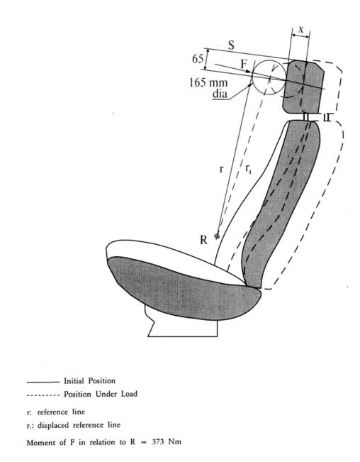
Figure 3 Determination of Dimension 'a' of Head Restraint Gaps
