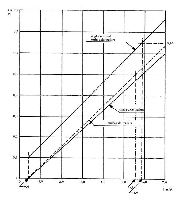
Compatibility of the braking rate of the trailer and the mean fully developed deceleration of the tractor/trailer combination (trailer laden and unladen)
