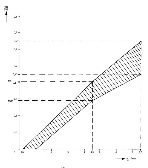
The relationship between the braking rate  $\frac{TR}{PR}$  and control line pressure for the laden and unladen condition is determined as follows:
