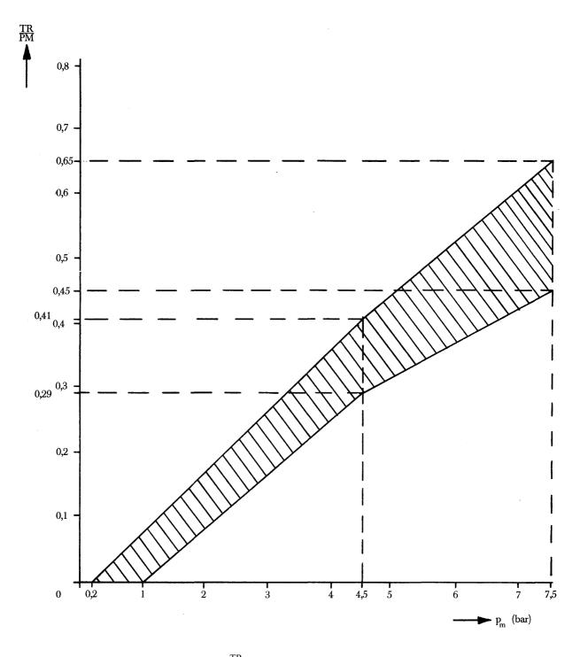
The relationship between the braking rate  $\frac{TR}{PR}$  and control line pressure for the laden and unladen condition is determined as follows:
