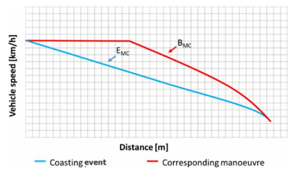
In order to comply with points (a)-(1) of Section 3.3, the same distance must be covered under the NEDC and mNEDC. Since the distance covered by the baseline vehicle in overrun is shorter than the distance covered during coasting by the eco-innovative vehicle, due to the higher deceleration rate of the baseline vehicle, the difference in the distance to be covered by the
