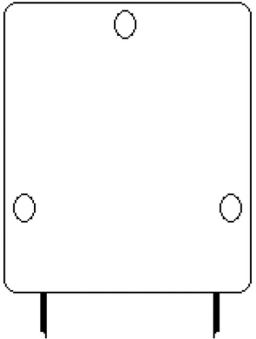
The front-end lights must optimise train detectability (marker lights), provide sufficient visibility for the train driver (head lights) by night and during low light conditions and must not dazzle the drivers of oncoming trains.
