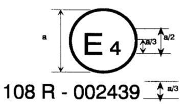
The above approval mark affixed to a retreaded tyre shows that the retreading production unit concerned has been approved in the Netherlands (E4) under approval number 108R002439, meeting the requirements of this Regulation in its original form (00).
