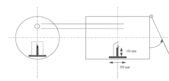
(f) the drum is laid on the ground or on a support at a spot where the temperature is between 15 °C and 25 °C; the product to be tested will be sprayed within the drum of roughly 200 dm<sup>3</sup> in which there will be a source of ignition.
