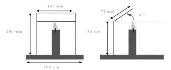
(e) the candle placed on the metal support shall be positioned midway between the two ends of the drum (see Figure below);
