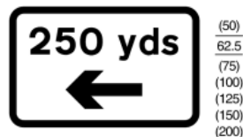
573 Distance and direction to hazard
