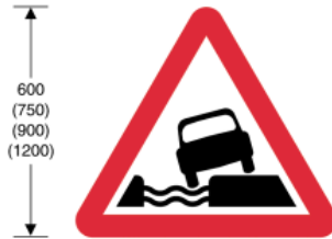
555.1 Water course alongside road ahead
