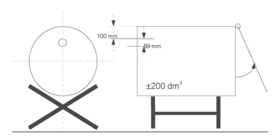
(d) on a  $200 \times 200$  mm metal support place a paraffin wax candle 20 to 40 mm in diameter and 100 mm high; the candle shall be replaced when having a height of less than 80 mm; the candle's flame is protected from the action of the spray by a 150 mm wide, 200 mm high deflector; this includes the plane inclined at 45° produced 150 mm from the base of the deflector (see Figure below);
