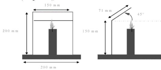
(e) the candle placed on the metal support shall be positioned midway between the two ends of the drum (see Figure below);
