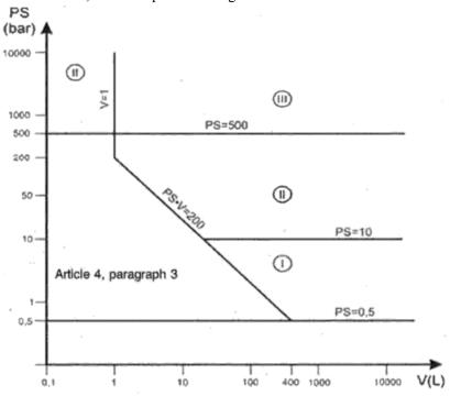
(d) (i) Table 4: Vessels for liquids having a vapour pressure at the maximum allowable temperature of not more than 0.5 bar above normal atmospheric pressure (1013 mbar) and, for fluids in Group 2 with a pressure PS greater than 10 bar and a product of PS and V greater than 10000 bar.L, or with a pressure PS greater than 1000 bar
