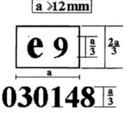
The exhaust system or component thereof bearing the above EC type-approval mark is a device which has been approved in Spain (e 9) pursuant to Directive 92/97/EEC (03) under the base approval number 0148.
