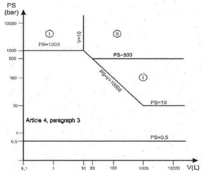
(ii) Exceptionally, assemblies intended for generating warm water at temperatures not greater than 110°C which are manually fed with solid fuels and have a PS.V, shall be subject either to a Type examination (Module B — design type) with respect to
