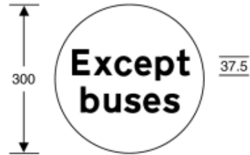
954.5 As diagram 954 where the signs are mounted in combination with light signals prescribed by regulation 33
