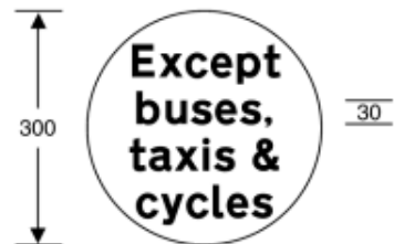
954.7 As diagram 954 applying to buses, taxis and pedal cycles where the signs are mounted in combination with light signals prescribed by regulation 33
