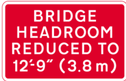
7014.1 Temporary or permanent reduction in bridge headroom ahead
