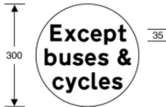
954.6 As diagram 954 applying to buses and pedal cycles where the signs are mounted in combination with light signals prescribed by regulation 33
