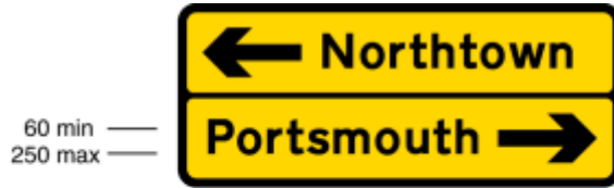
2705 Junction ahead leading to temporary diversion routes to the destinations shown
