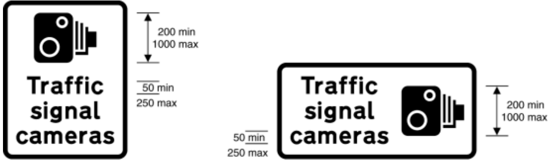
878 Area in which cameras are used to enforce traffic regulations (Alternative types)
