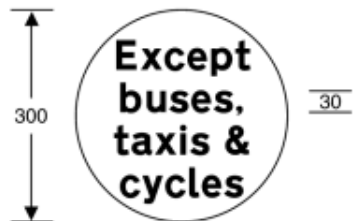
954.7 As diagram 954 applying to buses, taxis and pedal cycles where the signs are mounted in combination with light signals prescribed by regulation 33
