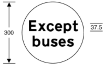
954.5 As diagram 954 where the signs are mounted in combination with light signals prescribed by regulation 33
