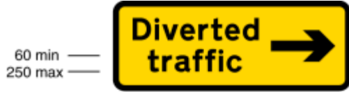
2703 Direction of temporary diversion route from junction ahead
