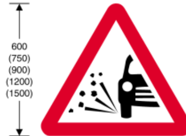
7009 Loose chippings on road ahead
