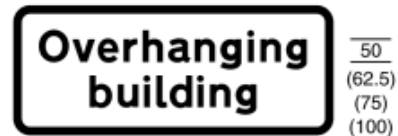
530.1 Reduced headroom over part of road due to overhanging building ahead
