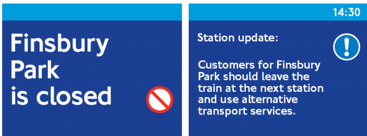
TFT layout showing additional 'real time' information about service disruption
