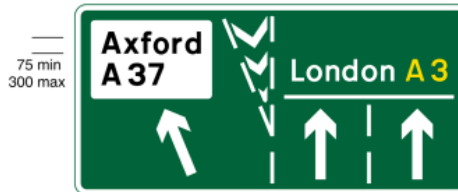
2018 Grade separated junction where the left hand lane of a primary route leaves the main carriageway of that route and leads to a non-primary route
