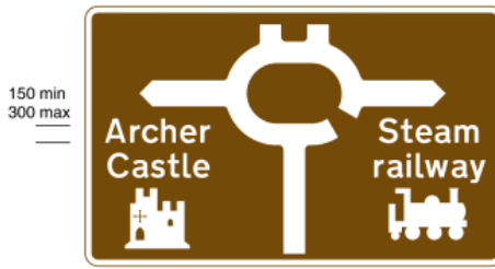
2925 Roundabout ahead leading from a motorway exit slip road to the tourist attractions shown
