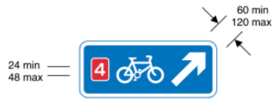
2601.1 Direction of a numbered route for pedal cycles forming part of a national cycle route network at a junction ahead
