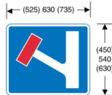
817 No through road for vehicular traffic in direction indicated from junction ahead
