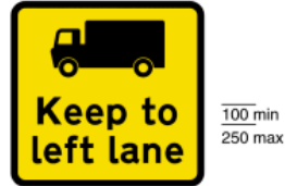
832.5 Goods vehicles should keep to left hand lane on approach to check point ahead
