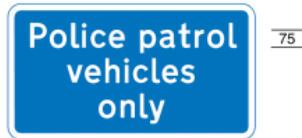
829.6 Waiting place at a lay-by or observation platform for police vehicles only
