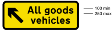
832.8 Goods vehicles should leave the main carriageway of a road on the approach to a goods vehicle check point
