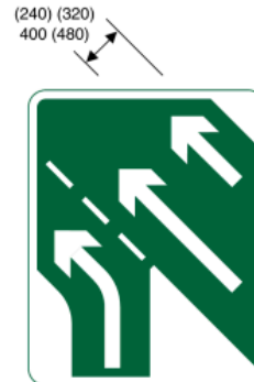
868.1 Additional traffic lanes joining from the right ahead
