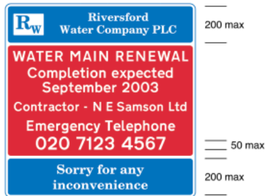
7008 Nature of street works, giving names of employer and contractor, emergency telephone number, and apology for inconvenience (Sign for pedestrians)
