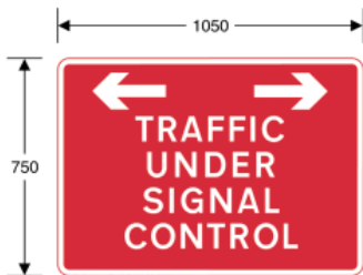
7021 Traffic on road ahead is being controlled by portable light signals (Indication to traffic joining that road)
