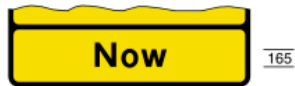
7272 Panel to appear at bottom of road works sign indicating that the change to the road layout indicated by signs shown in diagrams in item 3 of the table occurs at that point
