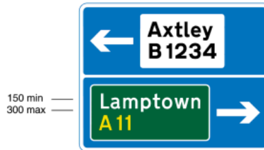
2913.2 Junction ahead leading from a motorway exit slip road to a primary and a non-primary route
