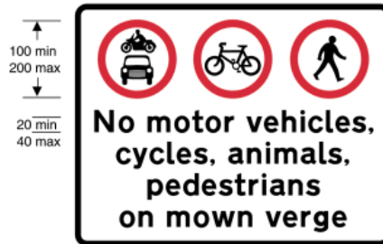
651 Use of verge maintained in mown or ornamental condition by specified traffic prohibited
