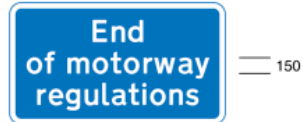
2932 Entrance to motorway service area, maintenance compound or similar facility contained within the length of a motorway and indicating that the Regulations referred to in the caption under diagram 2901 cease to apply at this point
