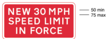
7032 Commencement point of a newly imposed 30mph speed limit which is contiguous to an existing 30mph speed limit
