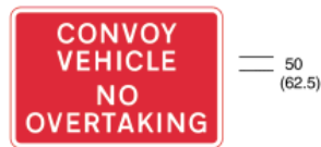
7029 Vehicular traffic must not overtake the vehicle used to escort other vehicles through road works
