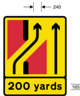
7214 Diversion of left hand lane from original carriageway to join right hand lane already diverted to the other carriageway
