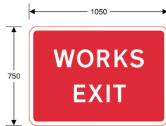
7302 Temporary exit from a construction or road works site
