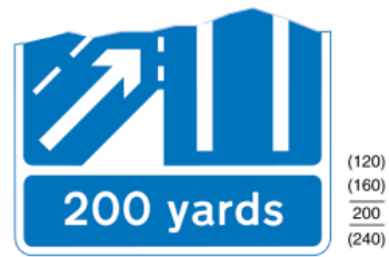
876 Distance to the change in the number of lanes indicated by the signs shown in diagrams 868 to 875
