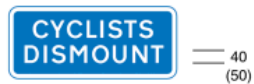
966 Pedal cyclists to dismount at the end of, or at a break in, a cycle lane, track or route
