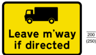
832.3 Goods vehicles may be directed to leave the motorway at a junction ahead
