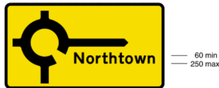
2706 Roundabout ahead leading to a temporary diversion route to the destination shown
