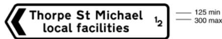
2309.1 Direction and distance to a small town or village offering the facilities indicated on the sign in diagram 2308.1
