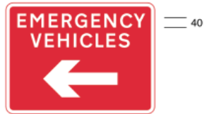
2708 Junction ahead leading to route for emergency vehicles to a temporary incident control point
