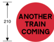
776 Another train or tramcar may be about to pass over the crossing
