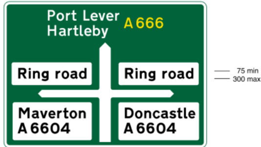
2033 Crossroads ahead between a primary route and a ring road which is a non-primary route
