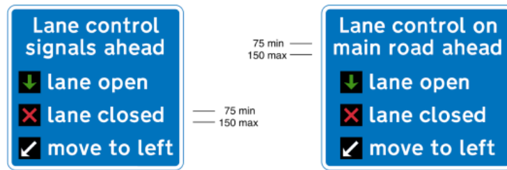
5010 Lane control light signals ahead as shown in diagrams 5001.1, 5003 and 5005 or diagrams 5001.2, 5003.1 and 5005.1
