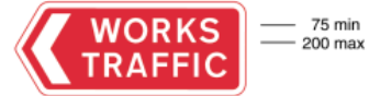
7305 Direction to be taken by road works or construction traffic at a junction or works entrance
