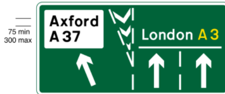
2018 Grade separated junction where the left hand lane of a primary route leaves the main carriageway of that route and leads to a non-primary route
