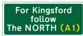
2034 Route to be followed at junction ahead for destinations that are not otherwise shown on signs for that junction
