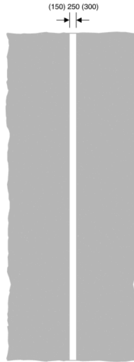
1049 Boundary of a bus lane, cycle lane, cycle track or route used by pedal cycles and pedestrians only. Where used in conjunction with the sign shown in diagram 957, the division of a route into that part reserved for pedal cycles and that part reserved for pedestrians
