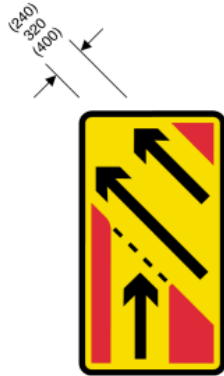
7253 Traffic joining main carriageway at a junction as part of temporary traffic management scheme; traffic on the main carriageway has priority
