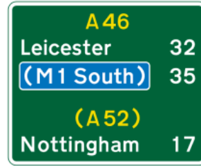
2030.1 Same as diagram 2030 but with the number of another primary route reached from that route and leading to a named destination
