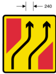
7237 Diversion of traffic from left and centre lanes to centre and right hand lanes
