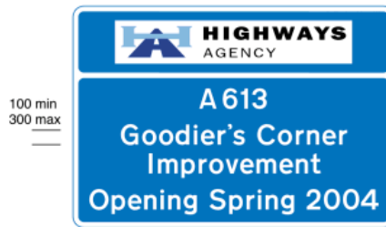
7007.1 Relevant particulars of major construction or improvement scheme being carried out on road ahead
