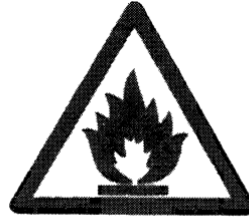
Flammable material or high temperature (a)
