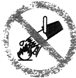
Do not extinguish with water
