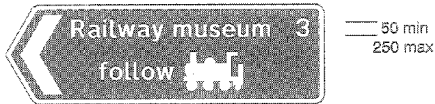
2207 Direction and distance to a tourist attraction where the route is subsequently indicated by a symbol
