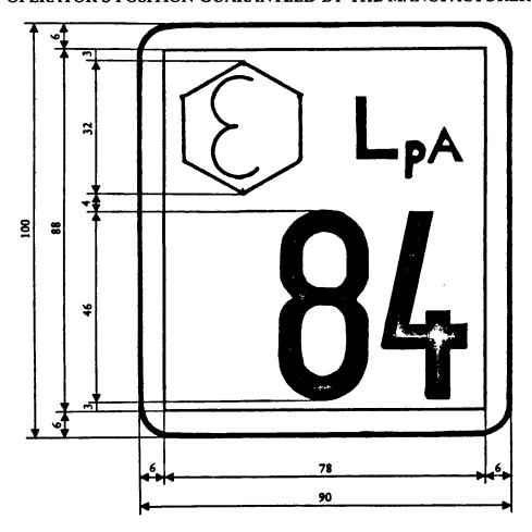
(Note: The figure 84 is for purposes of illustration and represents the sound pressure level as mentioned in regulation 6).
