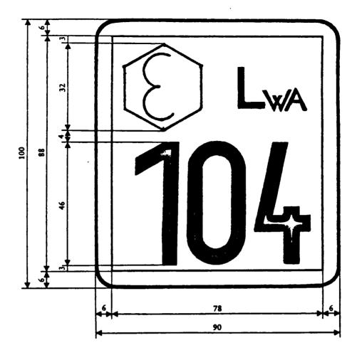
(Note: The figure 104 is for purposes of illustration and represents the sound power level as mentioned in regulation 6).
