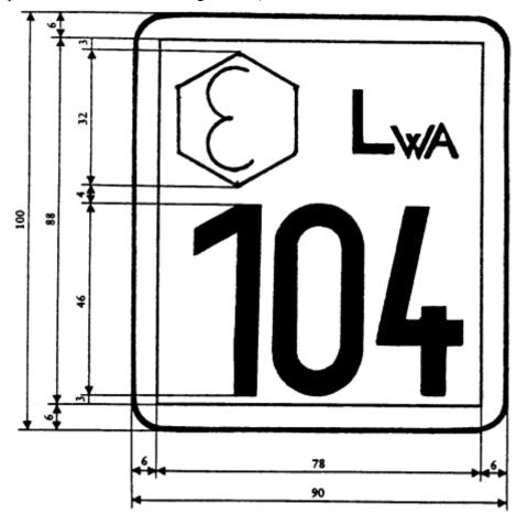
MODEL OF PLATE STATING THE SOUND PRESSURE LEVEL AT THE OPERATOR'S POSITION GUARANTEED BY THE MANUFACTURER MODEL OF PLATE STATING THE SOUND PRESSURE LEVEL AT THE OPERATOR'S POSITION GUARANTEED BY THE MANUFACTURER(Note: The figure 84 is for purposes of illustration and represents the sound pressure level as mentioned in regulation 6).
