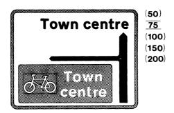
(Blue border; black lettering and route symbol on white background; cycle symbol and destination in white on a blue panel.) Same as 729 with variation for a road where the route for pedal cycles is different from the route for other vehicular traffic 729.3
