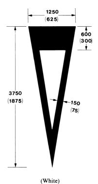
To indicate to vehicular traffic the approach to a road junction at or near which is placed the marking shown in diagram 1003 or both the marking shown in diagram 1003 and the sign shown in diagram 602.
