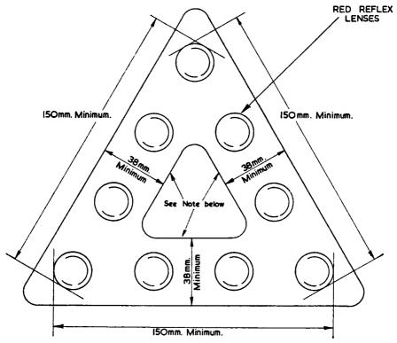
Note: The plate may be constructed without the central triangular space shown above.
