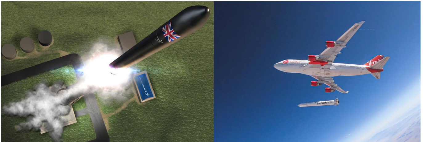
Figure 11: Artist's impression of Lockheed Martin vertical launch (left) and photo of Virgin Orbit carrier craft, Cosmic Girl, and launch vehicle, LauncherOne (right) 166
