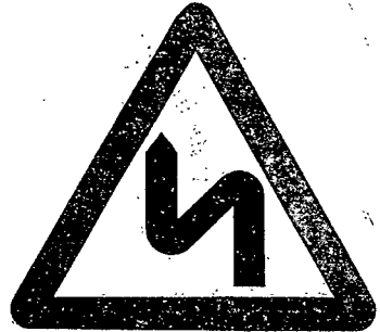
Double bend, first to the left Permitted variant: The symbol may be reversed 13
