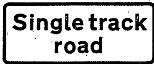
Road only wide enough for one line of vehicles Plate for use with signs in diagrams 16 and 17 19
