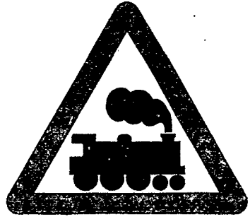
Level crossing without gate or barrier 31
