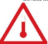
The background colour of the sign shall be white, and the colour of the border and the thermometer symbol shall be red.".
