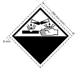
(e) comply with the measurements in the diagram except that larger measurements may be used in which case the measurements shall be increased proportionally.
