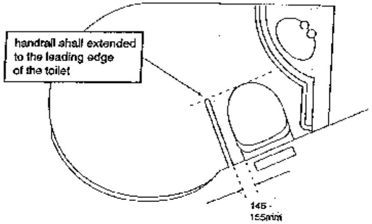
Diagram D1 - Hinged handrail
