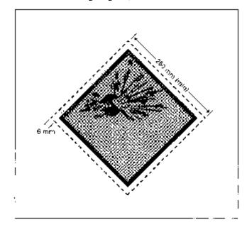
(b) comply with the measurements in the diagram, except that larger measurements, increased proportionally, may be used.
