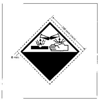
(b) comply with the measurements in the diagram except that larger measurements, increased proportionally, may be used.
