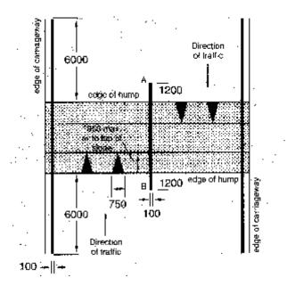
To indicate to vehicular traffic the presence of a flat top road hump extending across the whole width of a carriageway.
