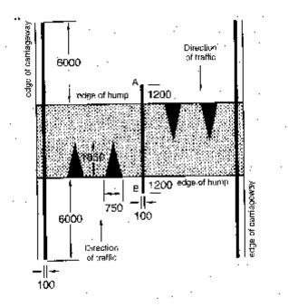
"To indicate to vehicular traffic the presence of a round top road hump extending across the whole width of the carriageway.
