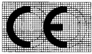
2. If the marking is reduced or enlarged, the proportions given in the above graduated drawing must be respected.
