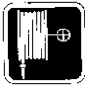
Fire hose Fire hose
