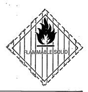
A substance which is liable to spontaneous heating under conditions encountered in conveyance by road or to heating in contact with air being then liable to catch fire.
