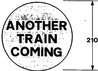
An electrically operated sign which, when illuminated so that the black letters of the legend appear against a red flashing background, indicates to road users the likely passage of another train over the level crossing.
