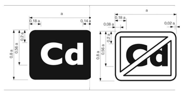
The dimension of 'a' shall be greater than 9 mm and the typeface to be used is 'Gill Sans'.
