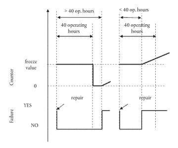
12.2. Figure 4.5 illustrates the operation of the activation and deactivation mechanisms when monitoring the reagent availability for four cases:
