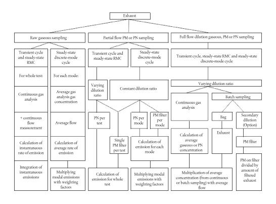
Note on Figure 6.2: The term 'Partial flow PM sampling' includes the partial flow dilution to extract only raw exhaust gas with constant or varying dilution ratio.
