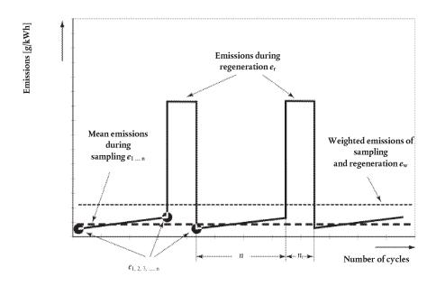
The average specific emission rate related to the test runs conducted according to points 6.6.2.1 or 6.6.2.2 [g/kWh or #/kWh] shall be weighted by means of equation (6-9) (see Figure 6.1):
