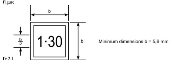
The above symbol shows that the corrected absorption coefficient is 1,30 m<sup>-1</sup>.
