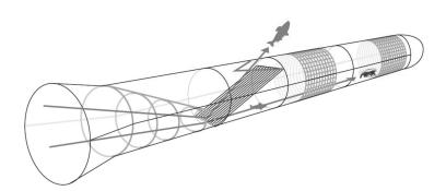
Schematic illustration of a size and species selective trawl. Entering fish is lead towards the trawl floor and grid via a leading funnel. Larger fish is then led out of the trawl by the grid while smaller fish and Norway lobster pass through the grid and enter the codend. The full square mesh codend enhance escapement of small fish and undersized Norway lobster.
