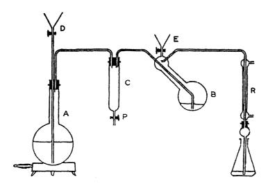
Tap-funnels P and E may be replaced by a plastic connector and a Mohr clamp.
