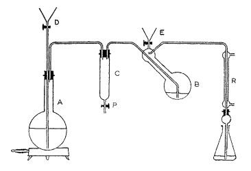
Tap-funnels P and E may be replaced by a plastic connector and a Mohr clamp.
